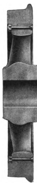
Figs. 1615-1616—Steel Tired Wheel with Cast Iron Spoke Center and Bolted Fastening Midvale Steel Company
