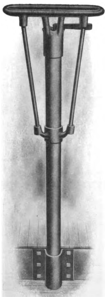
Fig. 668—Conductor's Control Stand for Pay-Within Car with Pneumatically Operated Door
