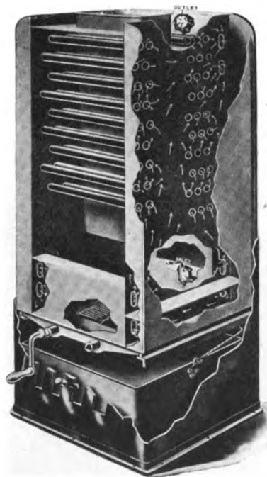
Fig. 1098—Sectional View of Cooper Pressed Steel Hot Water Car Heater The Cooper Heater Company
