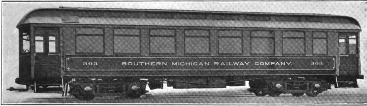
Fig. 118—Double-End Interurban Car with Steel Underframe St. Louis Car Company, Builder
