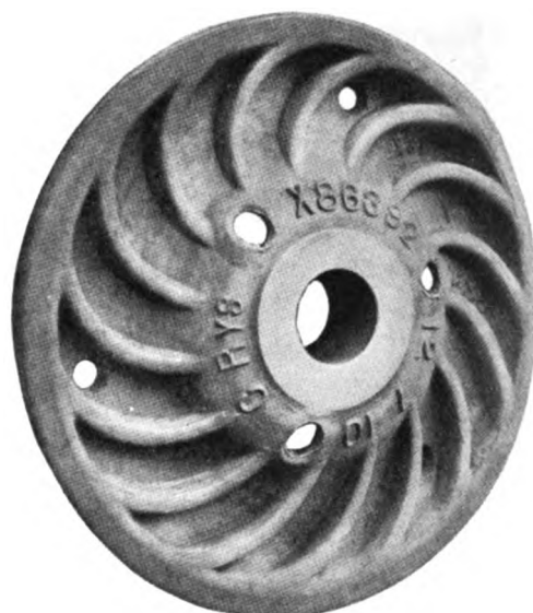
Fig. 1604—Back of Double Plate "F. C. S." Cast Iron Wheel Griffin Wheel Company
