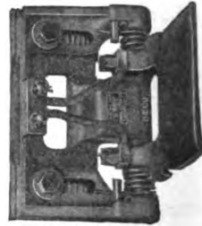
Figs. 1857-1858—Slipper Type Third-Rail Shoe for Underrunning Third Rail; Capacity, 800 Amperes General Electric Company
