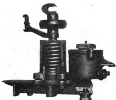
Fig. 1786—Cylinder and Magnet Valve of Unit Switch
