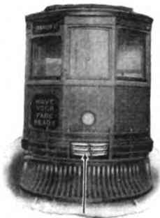
Combination Anti-Climber Draw Head Steel Casting Made to Any Size
