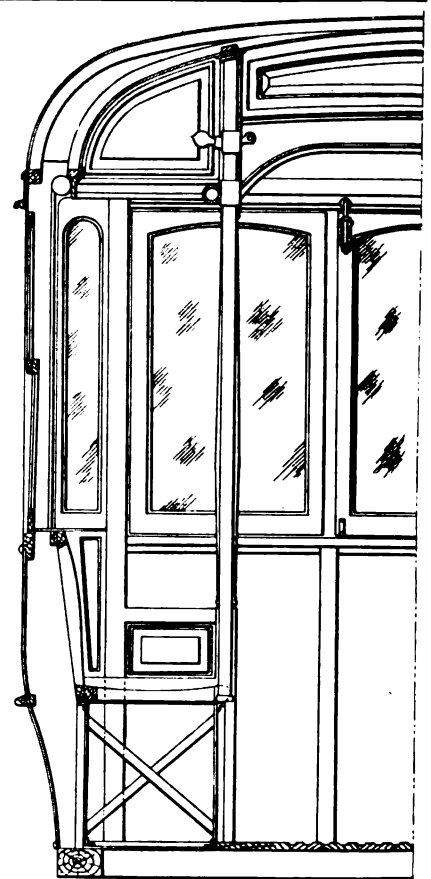
Fig. 263a—Half Cross-Section of Light Storage Battery Car Body J. P. Sjöberg & Co., Builders
