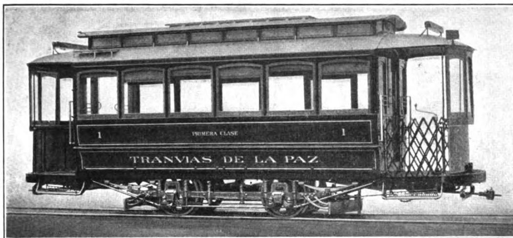
Fig. 1—Single-Truck, Double-End, Closed Car with Open Platforms and Portable Vestibules The J. G. Brill Company, Builder
