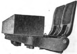
Figs. 1855-1856—Slipper Type Third-Rail Shoe for Overrunning Third Rail; Capacity, 2,000 Amperes General Electric Company
