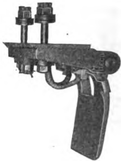
Figs. 1857-1858—Slipper Type Third-Rail Shoe for Underrunning Third Rail; Capacity, 800 Amperes General Electric Company
