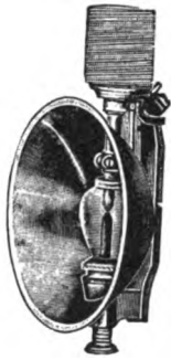
Figs. 1028-1029—Moshier Non-Metallic Circuit Electric Arc Headlight for Outside of Dasher
