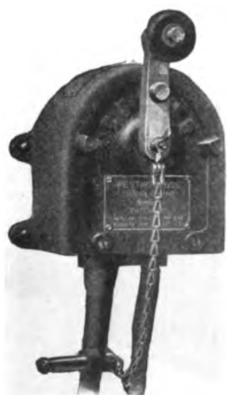
Fig. 1795—Master Controller for Type AB Electro-Pneumatic Multiple-Unit Control (277)
