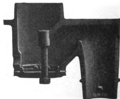
Fig. 1222—Sectional View of Pneu- matic Sander Trap
