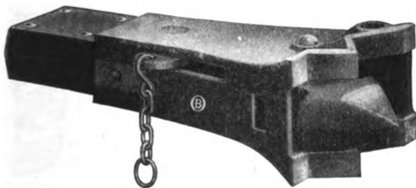
Fig. 625—Tomlinson Coupler Head for Attachment to Channel Bar Draft Stem
