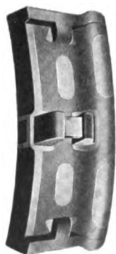
Fig. 1496—Steel Back Flanged Brake Shoe
