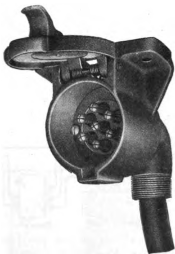
Fig. 1766—Coupler Socket for Train Line Control Wire Jumper
