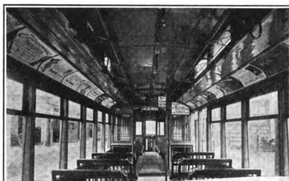
Fig. 87—Standard Double-Truck, Single-End, Combination Open and Closed Motor Car with Center Side Entrance; Denver City Tramway Company Woeber Carriage Company, Builder
